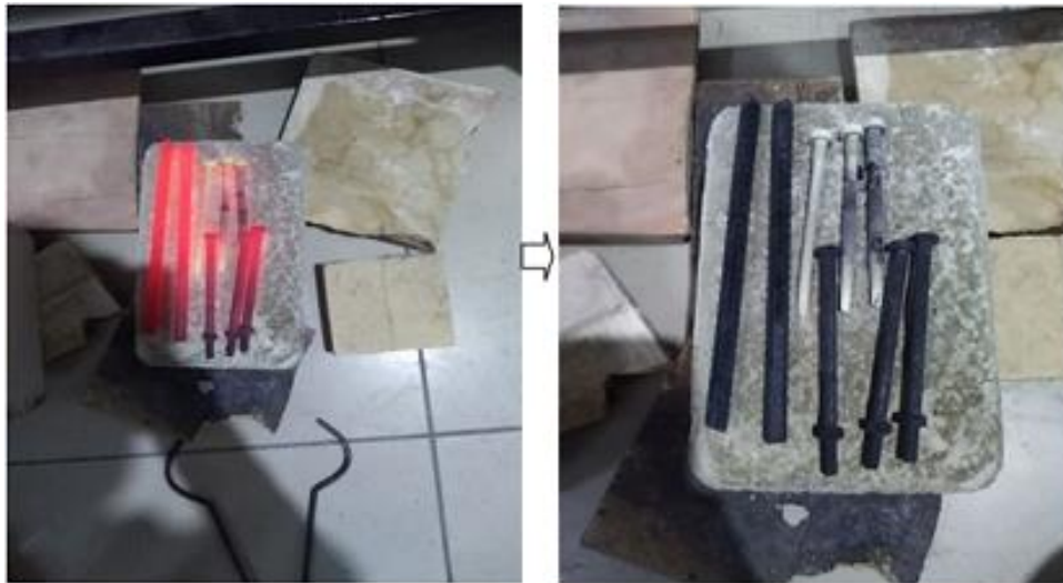
Fig. 4. Samples inside and outside the concrete that were left to cool in air.
