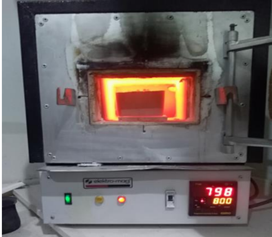
Fig. 3. Ash furnace providing desired temperatures.
