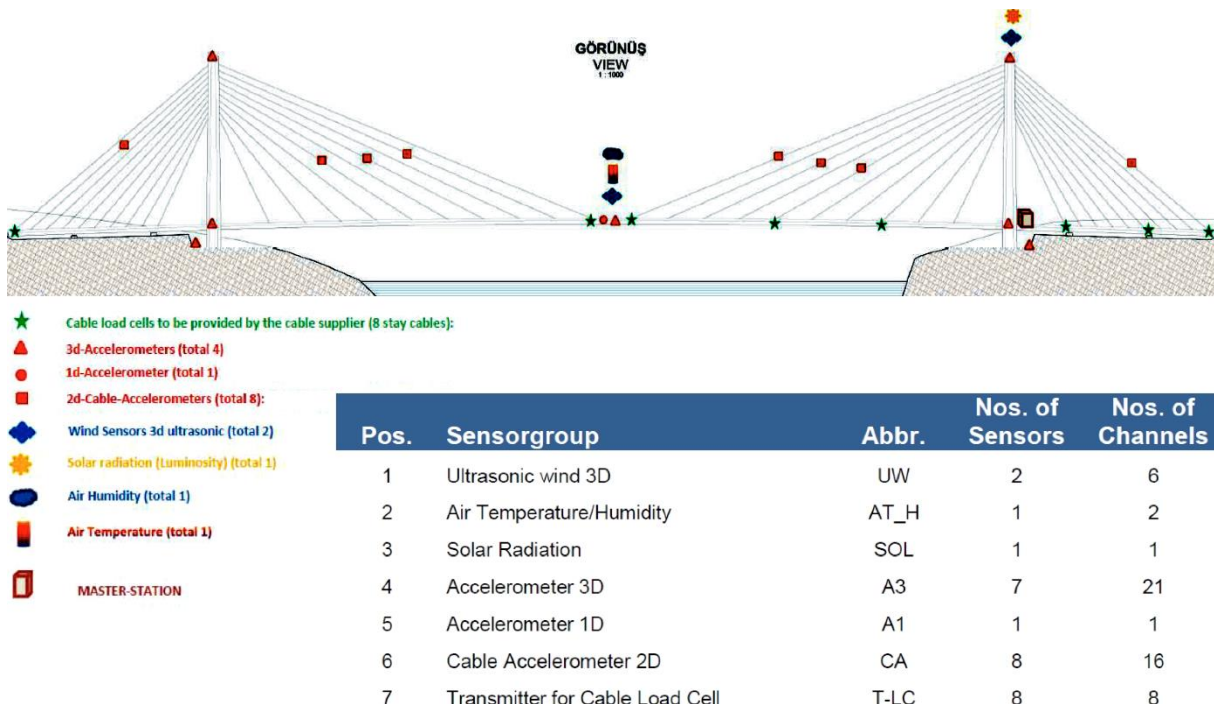
Fig. 2. The sensor types and locations in Nissibi Bridge (VCE, 2012).
