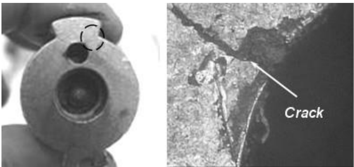
Fig. 11. Cracked torsional shaft of HKS.
