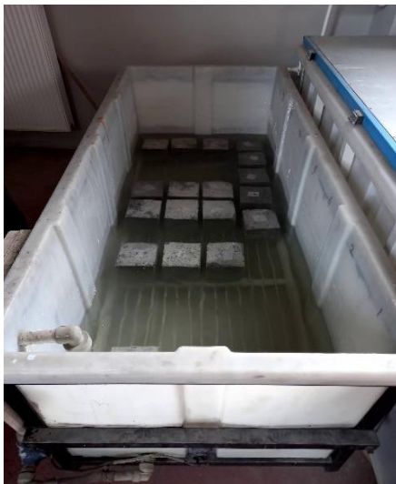
Fig. 6. Keeping the concrete samples in the water pool.
