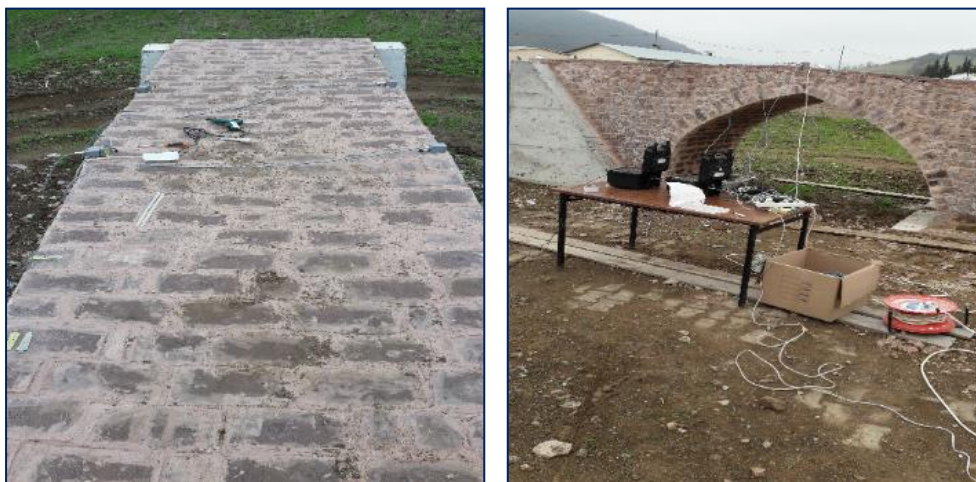
Fig. 7. Experimental application of reduced-scale masonry bridge.
