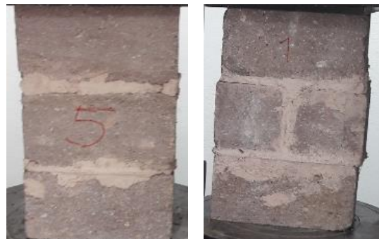
Fig. 3. Experimental assemblage samples with Khorasan mortar.
