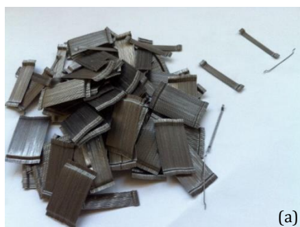
Fig. 1. (a) Polypropylene fibers; (b) steel fibers used for reinforced concrete.
