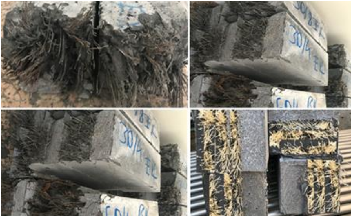
Fig. 6. Images of some SIFCON samples containing steel fiber and synthetic fiber after bending test.
