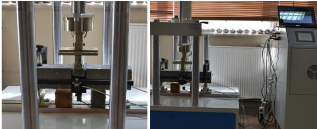
Fig. 5. Displacement controlled loading test device and bending test images.
