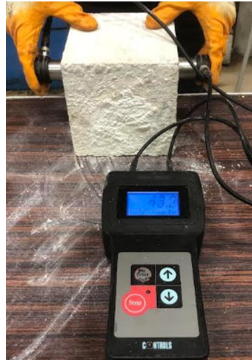
Fig. 4. Ultrasonic pulse velocity and mechanical tests.
