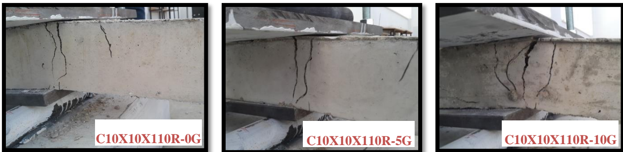
Fig. 11. Impact failure of cantilever column C10x10x110R-0G, C10x10x110R-5G and C10x10x110R in impact load.
