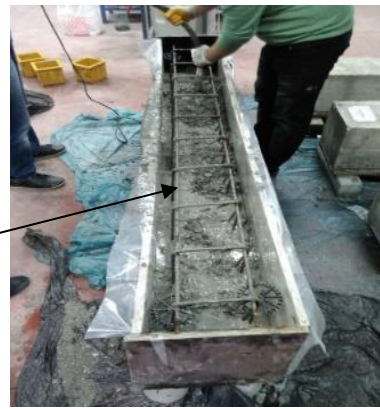
Fig. 3. Pouring the concrete material into the beam molds and performing the vibration process (Karalar 2020).
