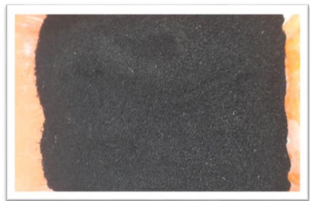
Fig. 1. 2-3 mm diameter crumbed rubber.
