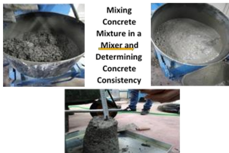
Fig. 1. Preparation of concrete material in the laboratory.
