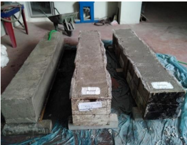
Fig. 4. View of prepared concrete beams (Karalar 2020).
