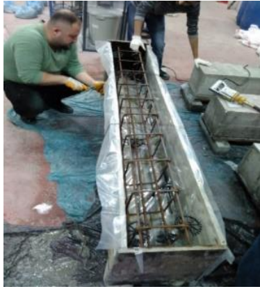
Fig. 2. Preparation of molds for concrete beams (Karalar 2020).
