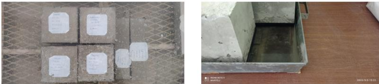
Fig. 5. Capillarity water absorption experiments.
