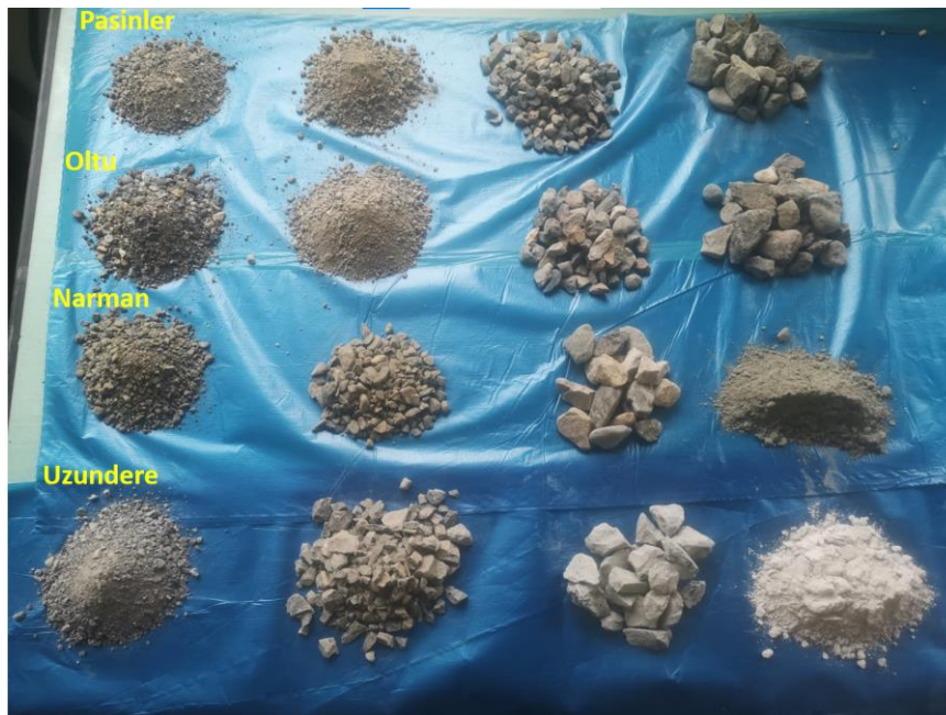
Fig. 2. Aggregates used in the concrete mix.
