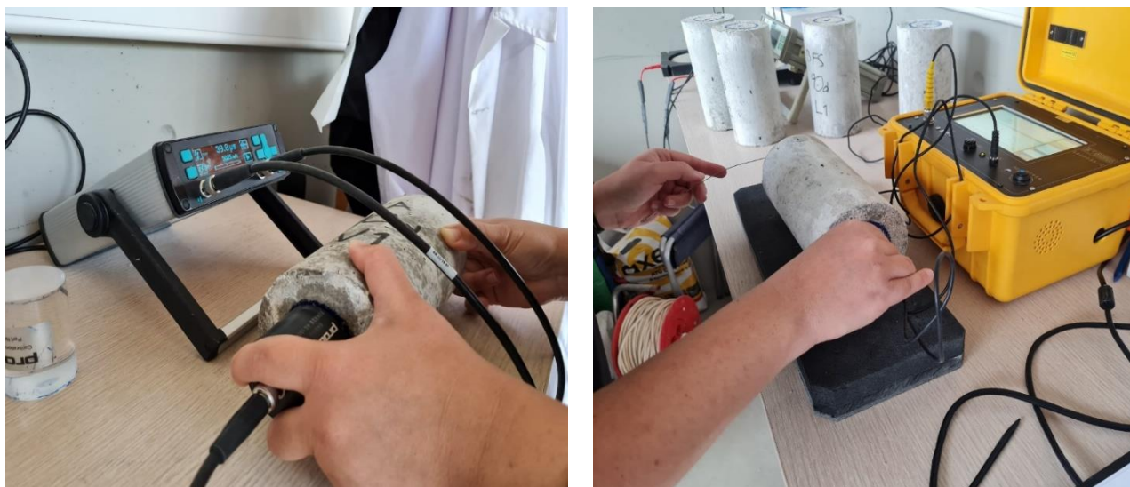
Fig. 4. Ultrasonic pulse velocity test and resonance frequency test.
