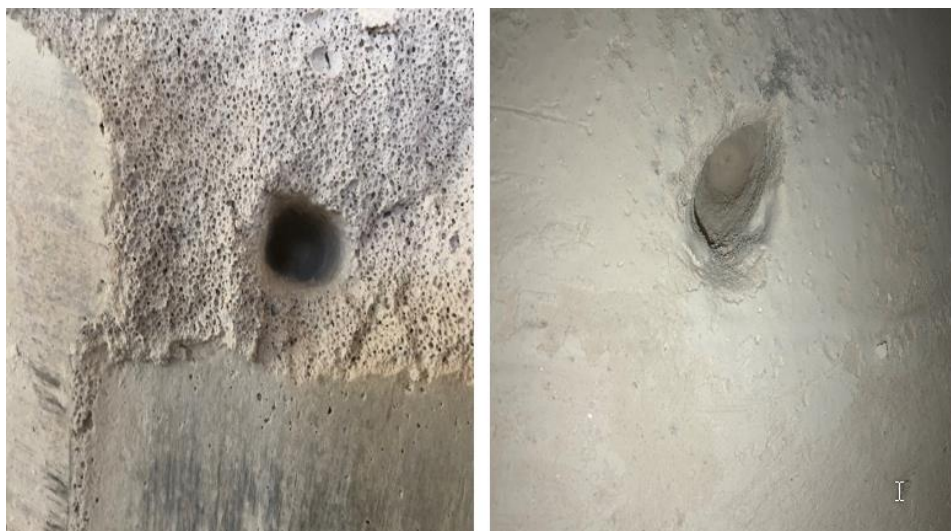
Fig. 10. Effect of shots fired on starch coated aerated concrete.
