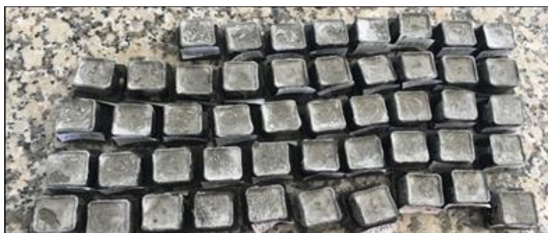
Fig. 2. Paste samples removed from the climate cabinet after 3 days.
