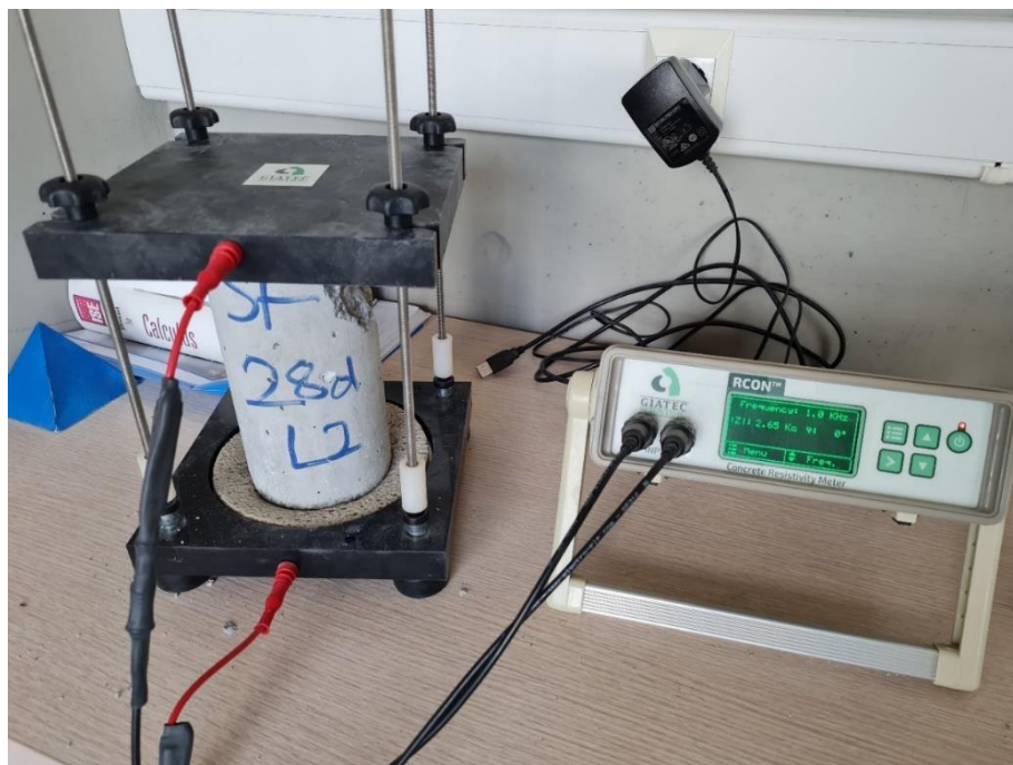
Fig. 3. Electrical resistivity test.
