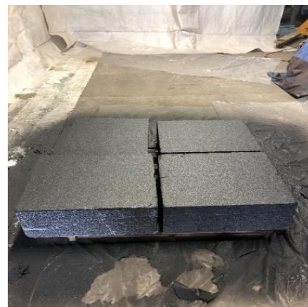
Fig. 2. Monolithic elastomer polyurea applied on the aerated concrete surface.
