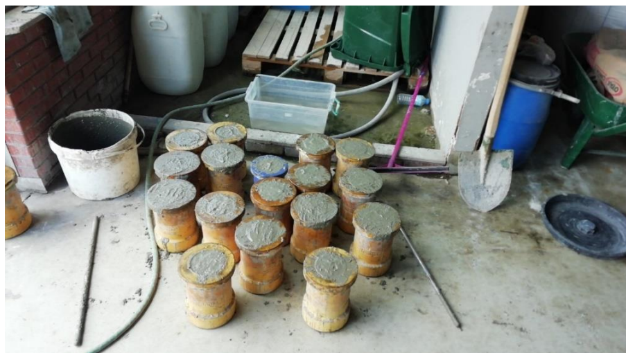
Fig. 1. Cylindrical concrete specimens.
