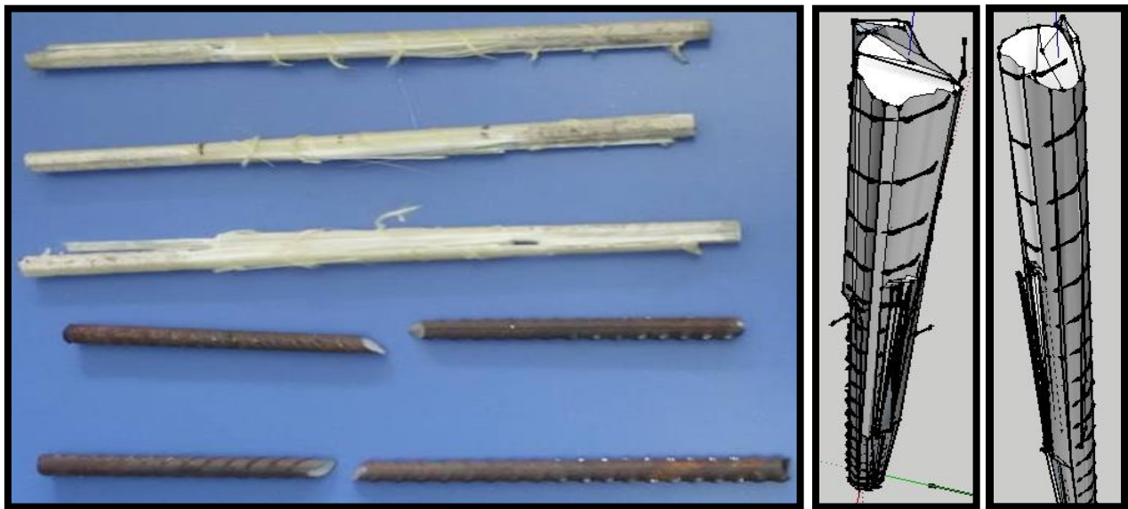
Fig. 8. Rupture patterns for S420 and GFRP bars.
