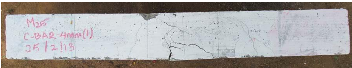
Fig. 33. Failure pattern of beams reinforced with diamond rib HYSD rebars.
