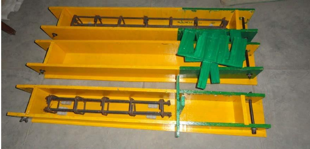
Fig. 5. View of fabricated moulds.
