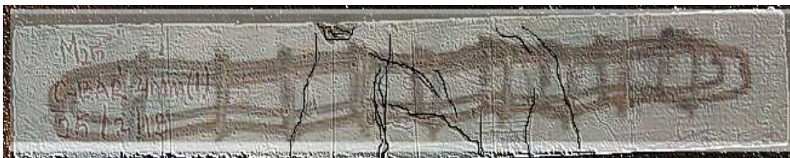
Fig. 34. Failure pattern of PSWC rebar (4mm deformation) reinforced beam.
