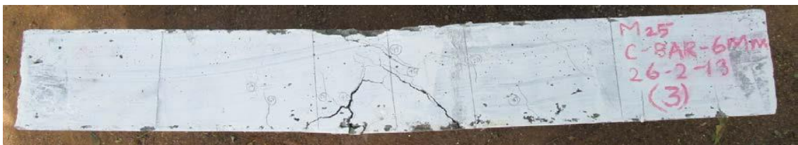
Fig. 34. Failure pattern of PSWC rebar (4mm deformation) reinforced beam.
