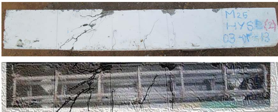
Fig. 31. Failure pattern of beams reinforced with spiral rib HYSD rebars.
