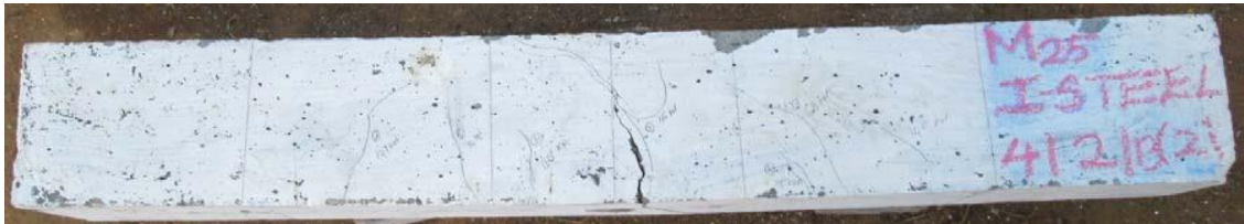
Fig. 32. Failure pattern of beams reinforced with mild steel rebars.
