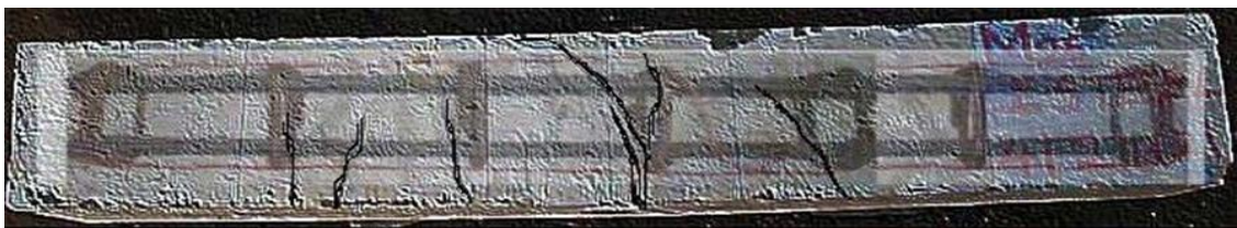
Fig. 33. Failure pattern of beams reinforced with diamond rib HYSD rebars.
