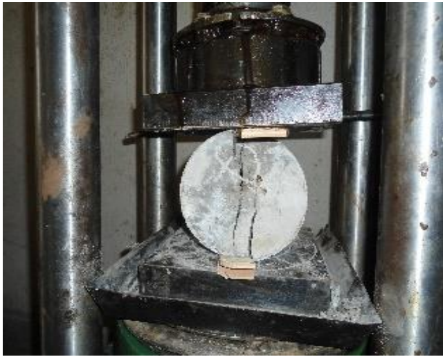
Fig. 4. Tensile strength test.
