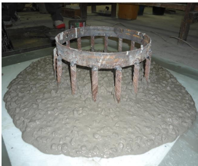
Fig. 7. J-Ring flow spread.
