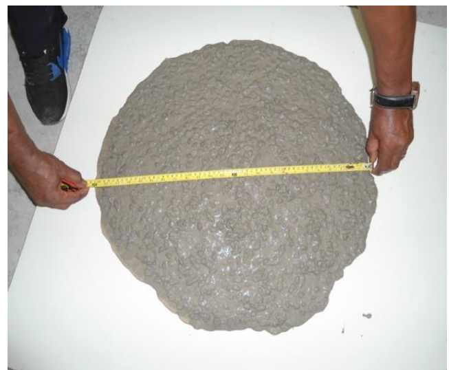
Fig. 8. Slump flow spread.
