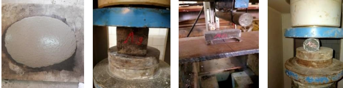
Fig. 2. Testing: Slump flow test; Compressive strength test; Flexural strength test; Splitting tensile strength test.
