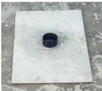
Fig. 4. The spread diameter test.
