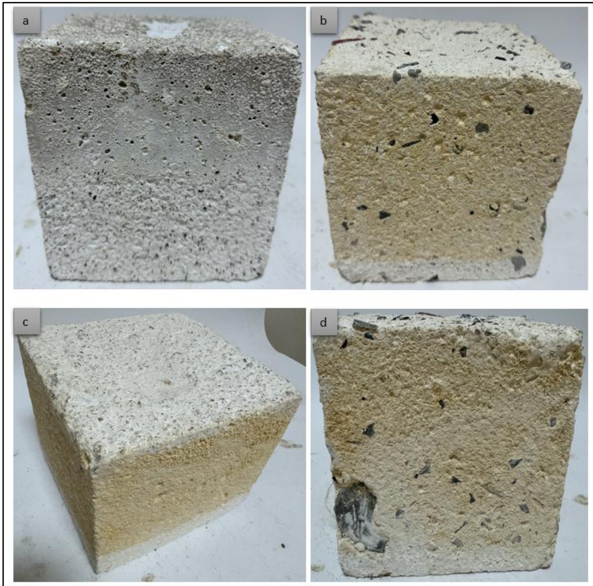
Fig. 7. Images of concretes exposed to acid attack for 90 days: (a) 5% waste rubber powder added concrete (P5E0/90); (b) 5% waste rubber powder and 5% e-waste added concrete (P5E5/90); (c) Control concrete (C/90); (d) 10% e-waste added concrete (P0E10/90).
