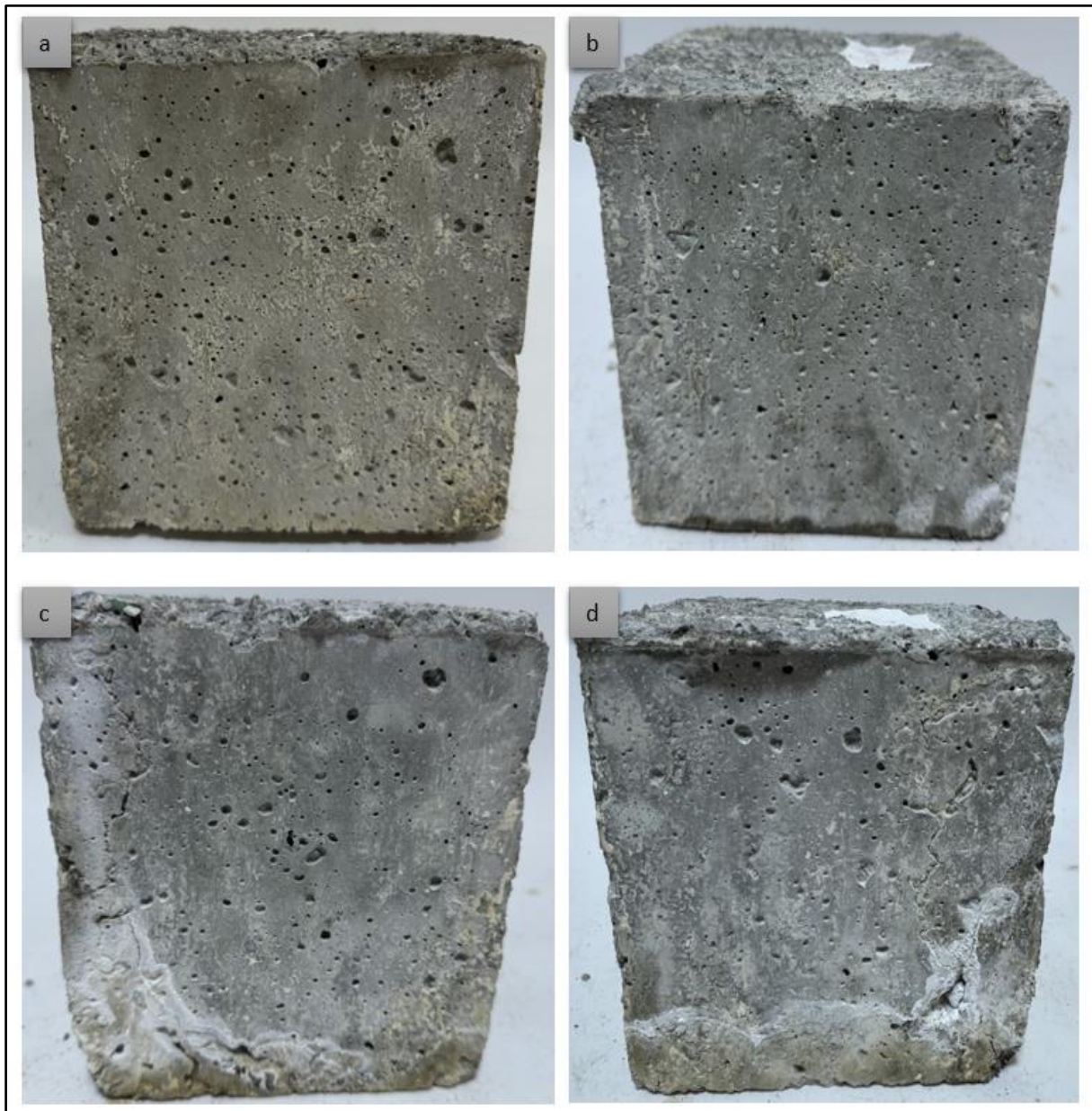
Fig. 10. Images of concretes exposed to sulfate attack for 90 days: (a) 5% waste rubber powder and 10% e-waste added concrete (P5E10/90); (b) 5% waste rubber powder and 5% e-waste added concrete (P5E5/90); (c) 5% e-waste added concrete (P0E5/90); (d) 10% e-waste added concrete (P0E10/90).
