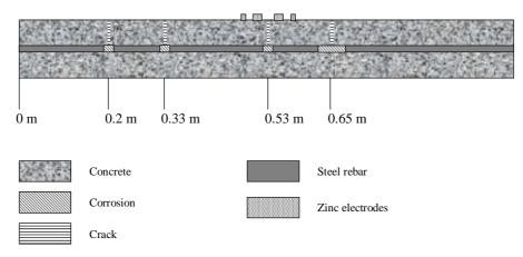
Figure 2. Concrete model, used for FEA with the crack locations
