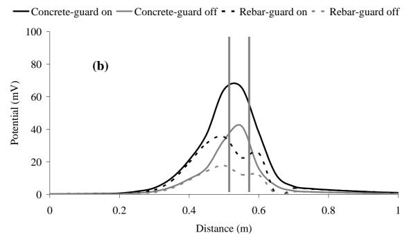
Figure 3. The current density distribution on the steel rebar and the polarization potential distribution on the steel rebar and concrete: (a) rings are on top of the crack location and (b) rings are not on top of the crack location. The vertical grey lines represent the position of the assumed measured area (70 mm)
