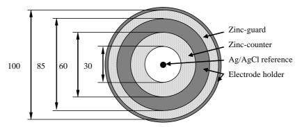
Figure 1. Schematic illustration of the instrument (i.e. GalvaPulse <sup>TM</sup>) using guard ring to limit the polarized area while performing the corrosion measurement.
