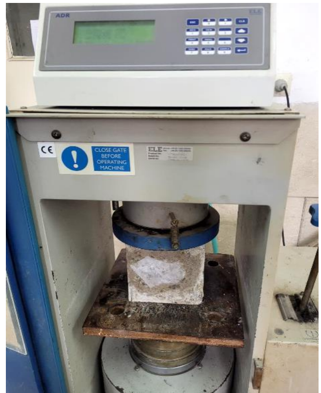
Fig. 7. Execution of the compressive strength test on a cubic specimen.
