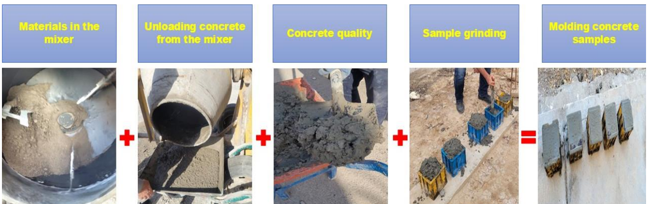
Fig. 4. Heavyweight concrete fabrication stages.
