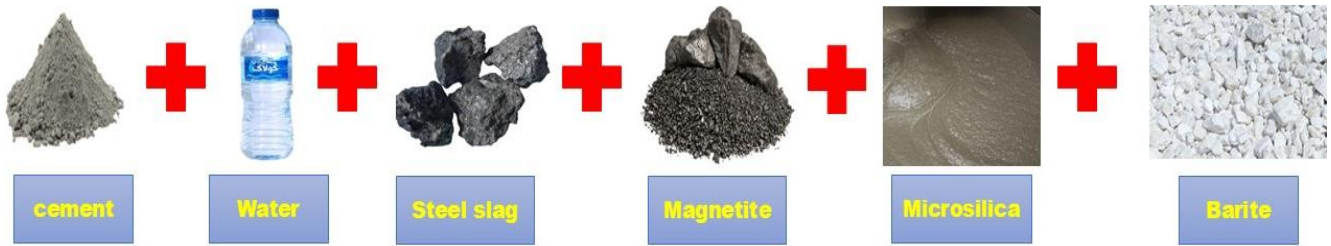
Fig. 3. Components of heavyweight concrete.
