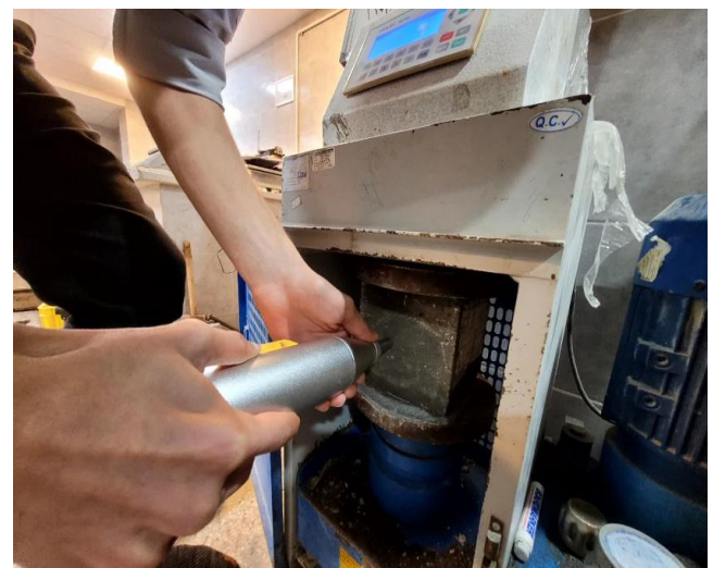
Fig. 6. Conducting the Schmidt hammer test on the cubic specimen.
