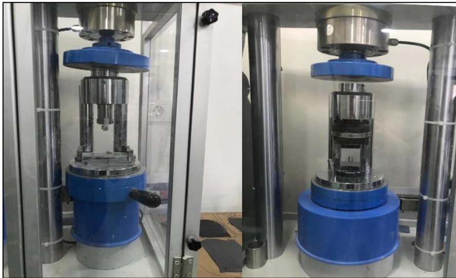
Fig. 9. Flexural and compressive strength test setup.
