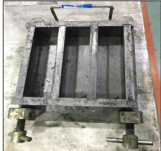
Fig. 5. Prism mold demonstration.
