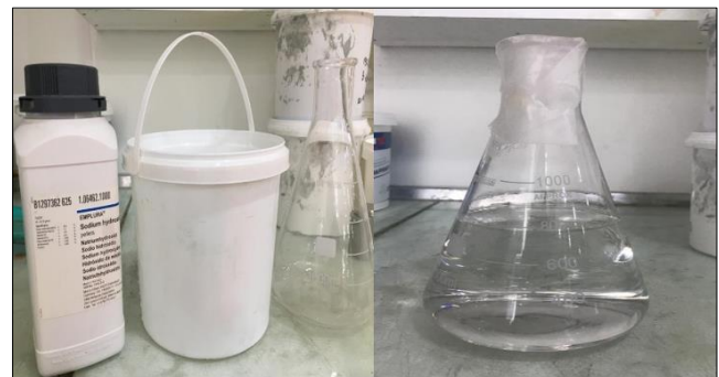
Fig. 3. Preparation of 8M sodium hydroxide solution.
