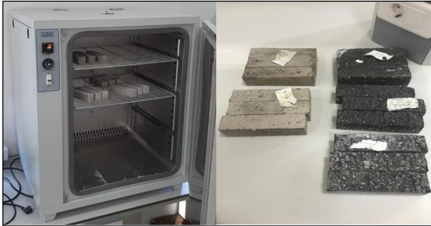
Fig. 8. 7-day specimen samples cured in 65 °C oven temperature.
