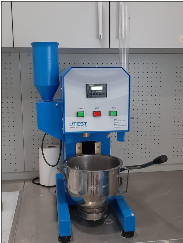
Fig. 4. Automatic programmable mortar mixer.
