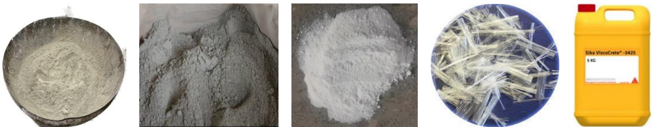
Fig. 1. Materials: Silica fume; Fly ash; Nano-silica; Polypropylene Fiber300–e3; Super-plasticizer.
