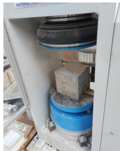
Fig. 5. The compressive strength test.
