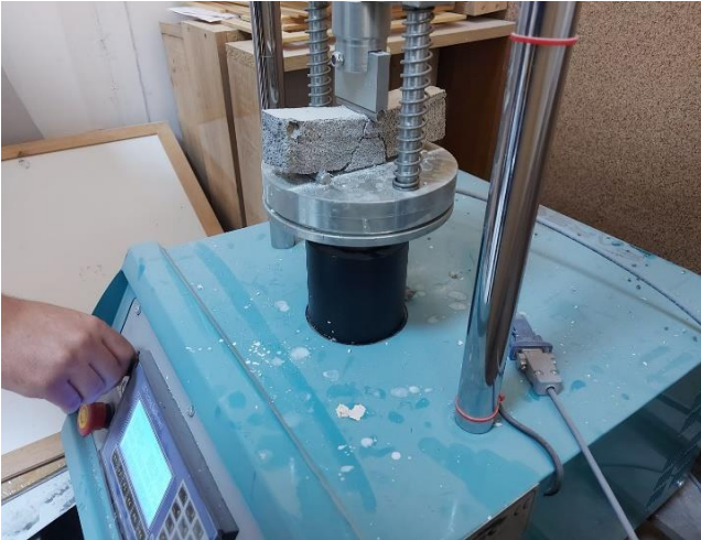
Fig. 6. The flexural strength test.
