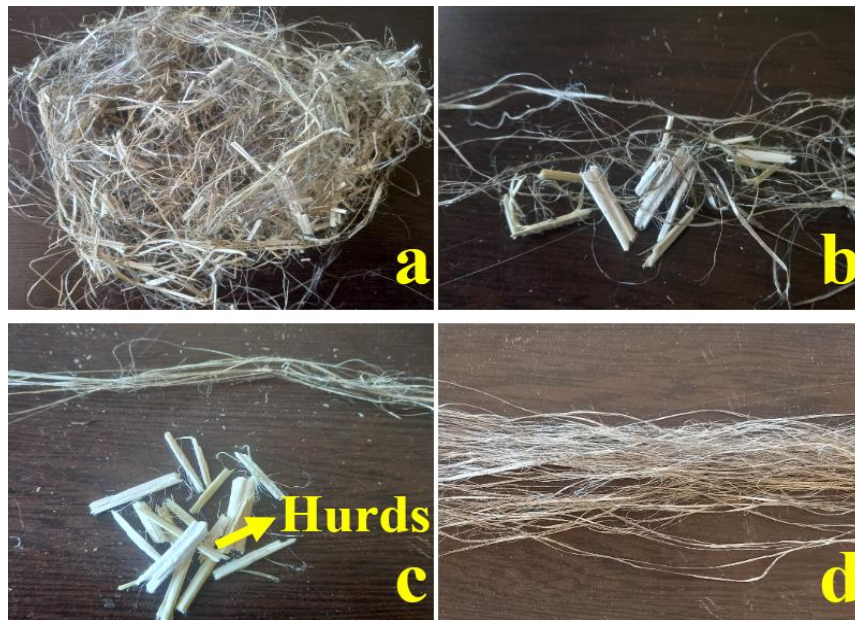
Fig. 1. Preparation of hemp fibers: (a),(b) Hemp fibers with hurds; (c) Cleaning fibers from hurds; (d) Hemp fibers before cutting.
