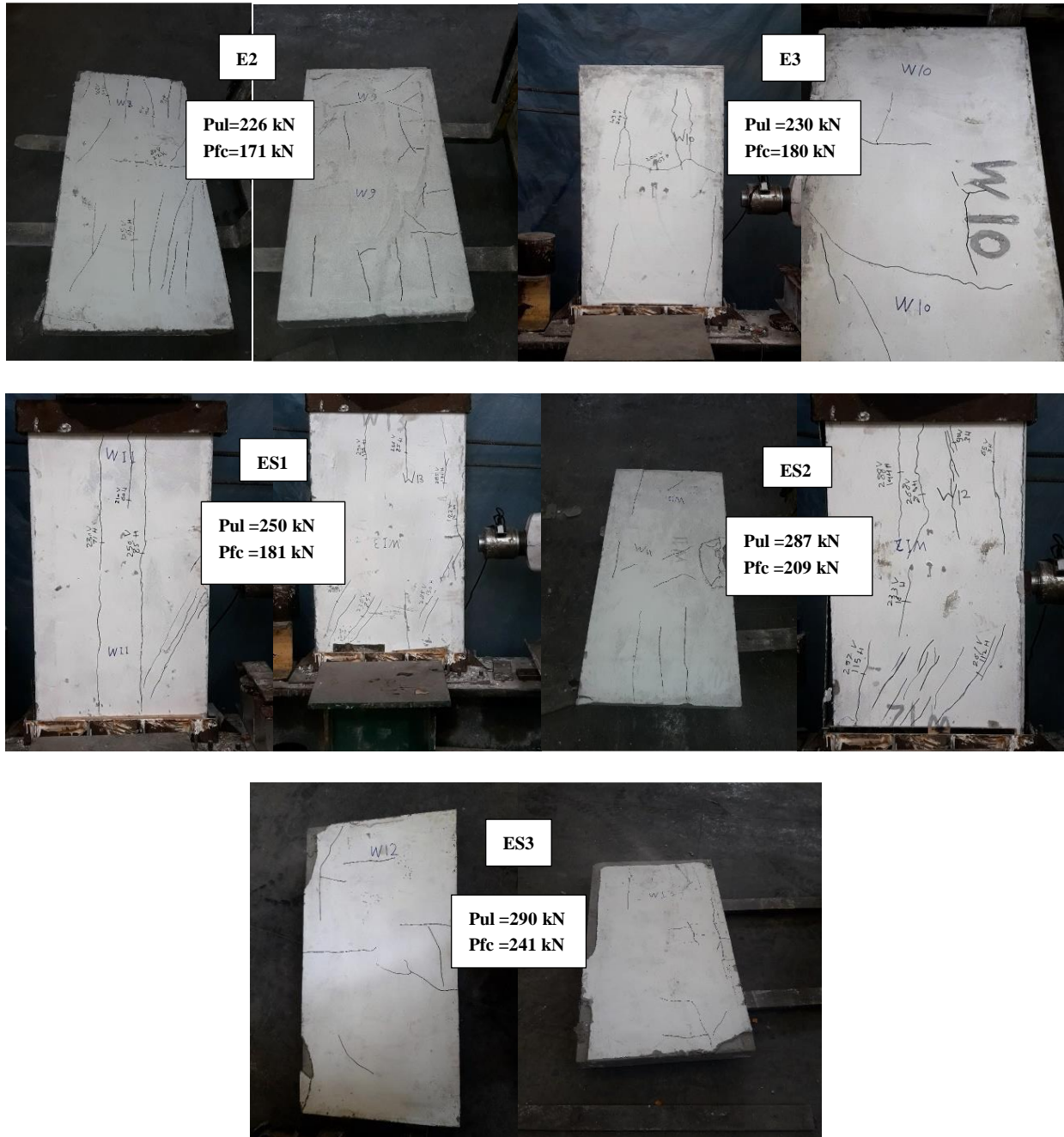
Fig. 27. Crack patterns of the wall.
