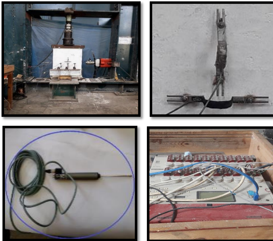
Fig. 8(a). Test set up and data logger unit used for the tests (TDS-150).
