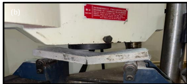
Fig. 17. Modes of failure under flexural load: (a) Normal LFC; (b) LFC with PP fiber.
