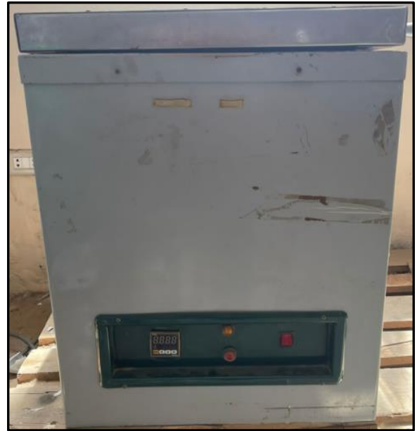
Fig. 3. Electric furnace used in this research.
