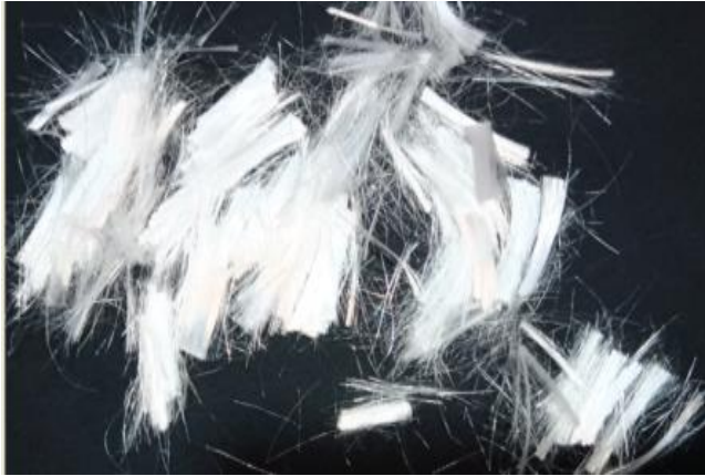
Fig. 1. Polypropylene fibers used in this research.
