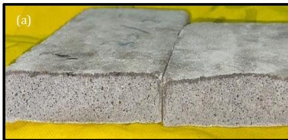
Fig. 17. Modes of failure under flexural load: (a) Normal LFC; (b) LFC with PP fiber.
