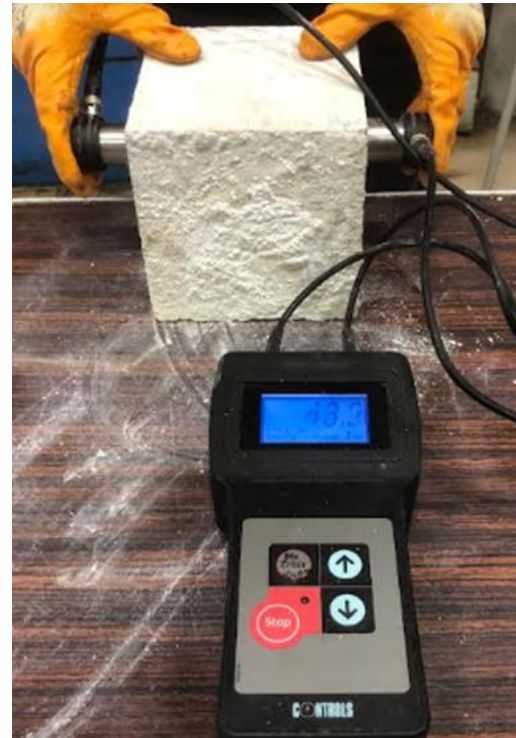
Fig. 4. Ultrasonic pulse velocity and mechanical tests.
