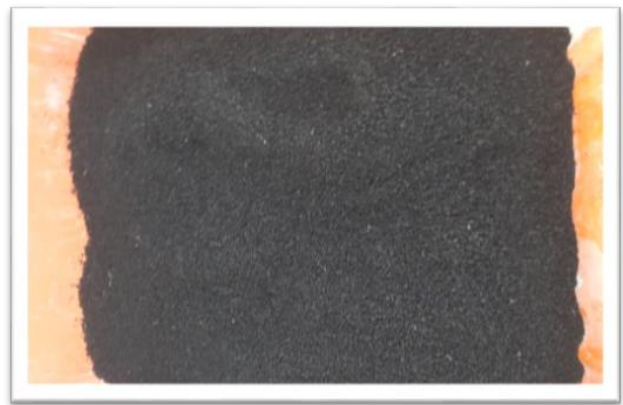
Fig. 1. 2-3 mm diameter crumbed rubber.
