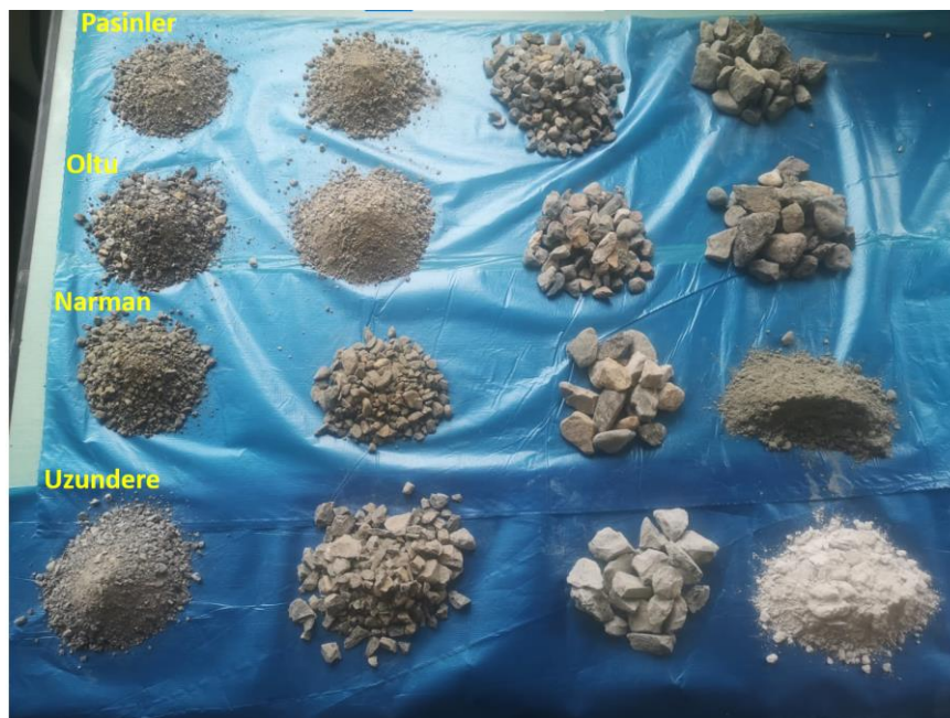
Fig. 2. Aggregates used in the concrete mix.
