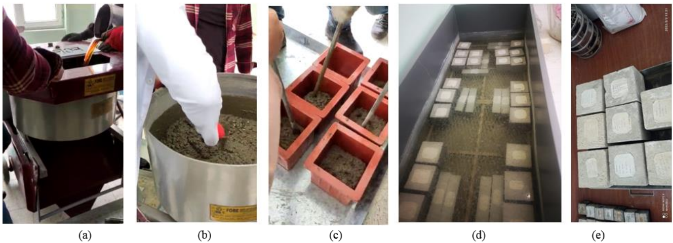
Fig. 3. Production stages of the concrete samples: a) Preparing the mixture in the mixer; b) Removing the mixture from the mixer; c) Molding the prepared mixture; d) Keeping the concrete samples in the curing environment; e) Concrete samples whose production has been completed.
