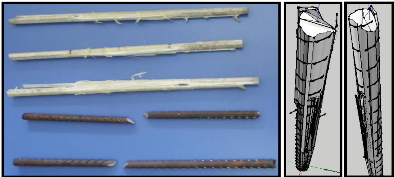
Fig. 8. Rupture patterns for S420 and GFRP bars.
