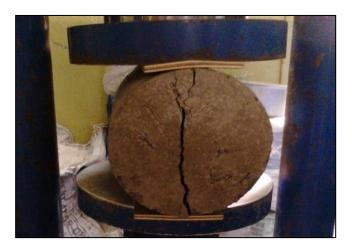
Fig. 1. Tensile strength test.
