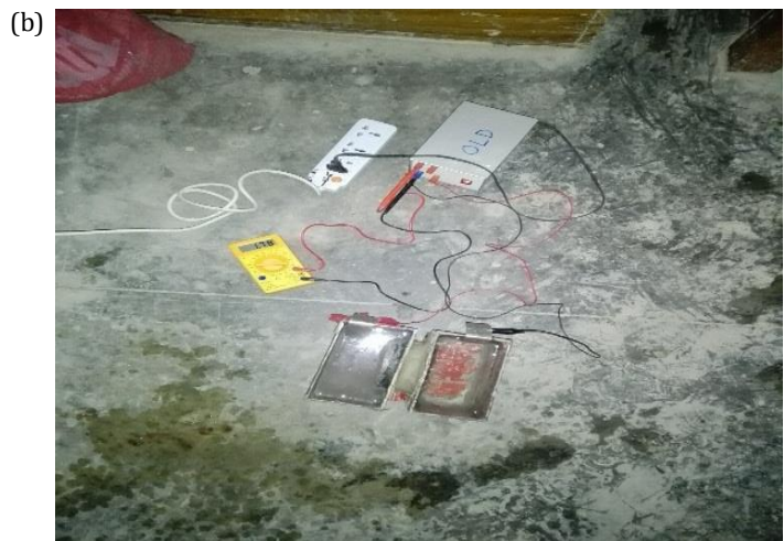
Fig. 3. (a) Experimental setup of chloride permeability test; (b) Practical set up of chloride permeability test.
