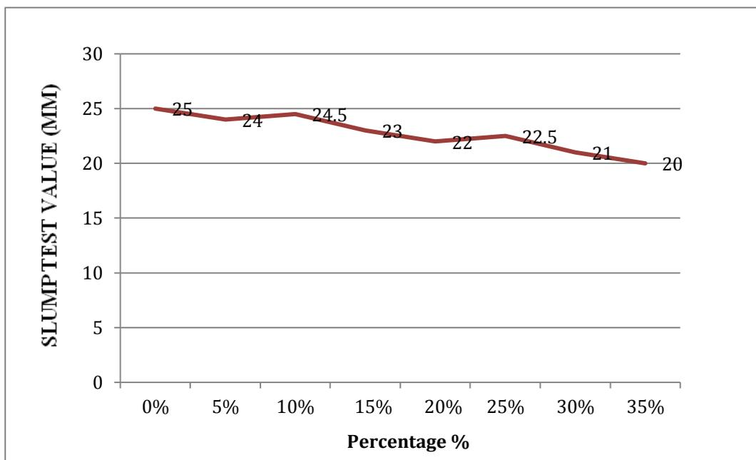
Fig. 4. Slump test values for different percentages.
