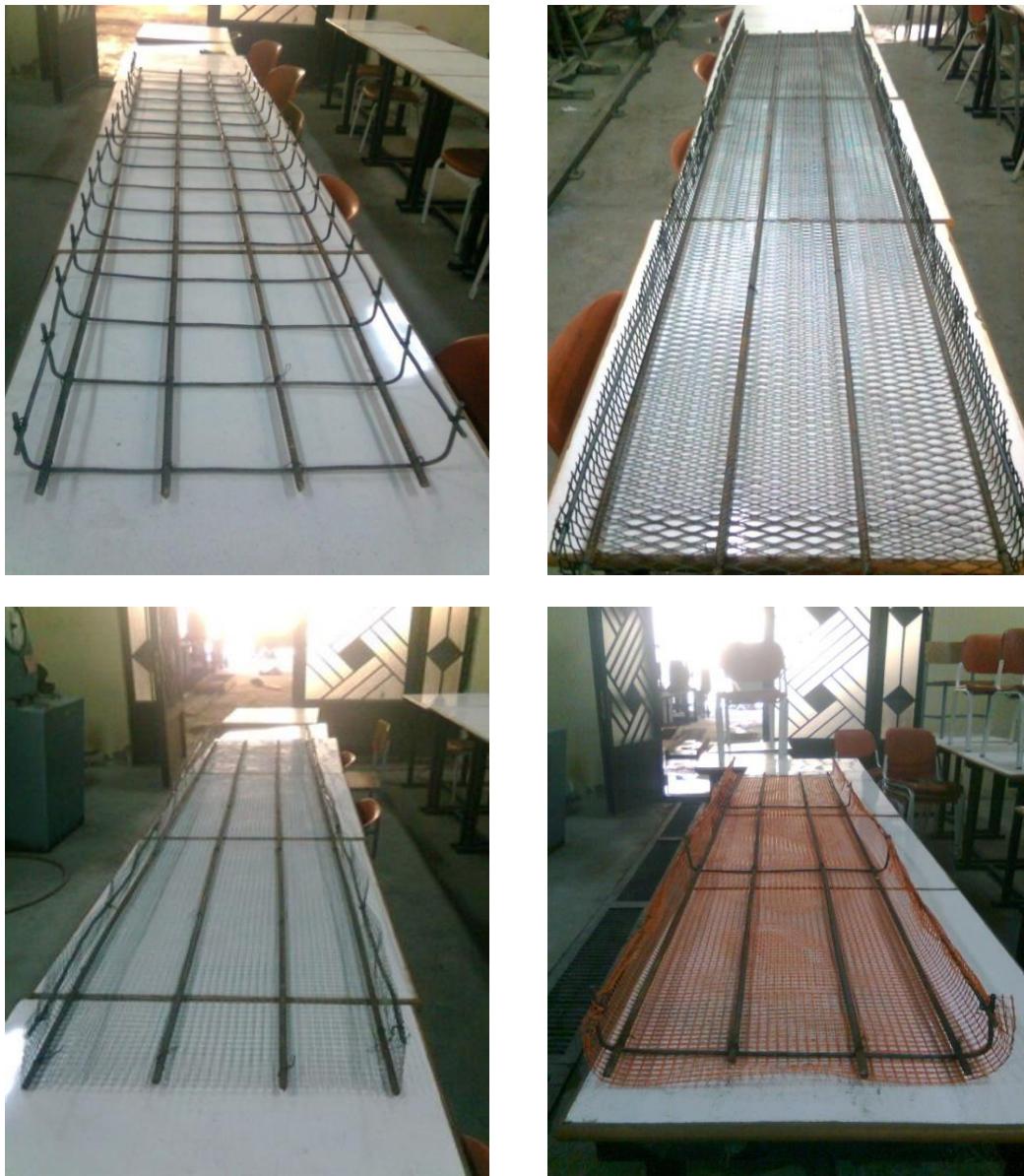
Fig. 3. Reinforcement configuration of U shape slabs.
