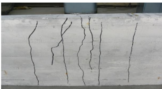
Fig. 26. Crack patterns of all tested slabs.
