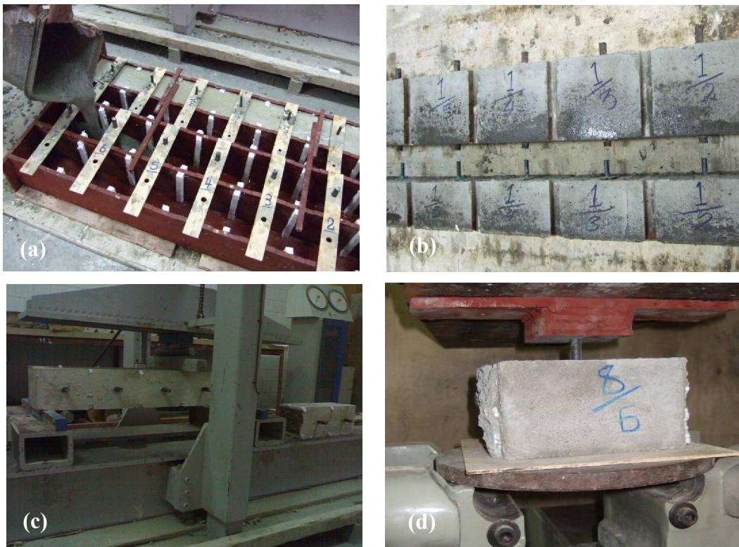
Fig. 4. Preparation and testing of push-out test specimens
