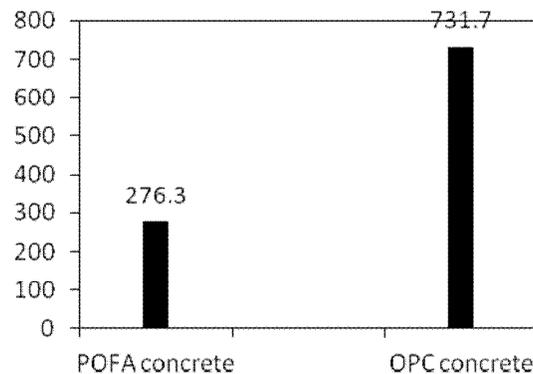
Figure 3: RCPT test results
