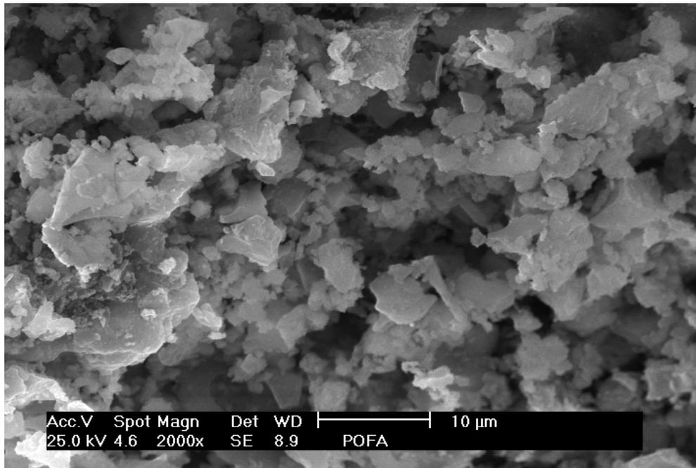
Figure 1: Scanning electron microscopy (SEM) of POFA
