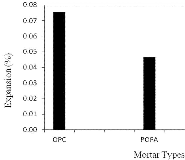
Figure 5: Expansion of mortar immersed in 5 % Na<sub>2</sub>SO<sub>4</sub> for 15 weeks.
