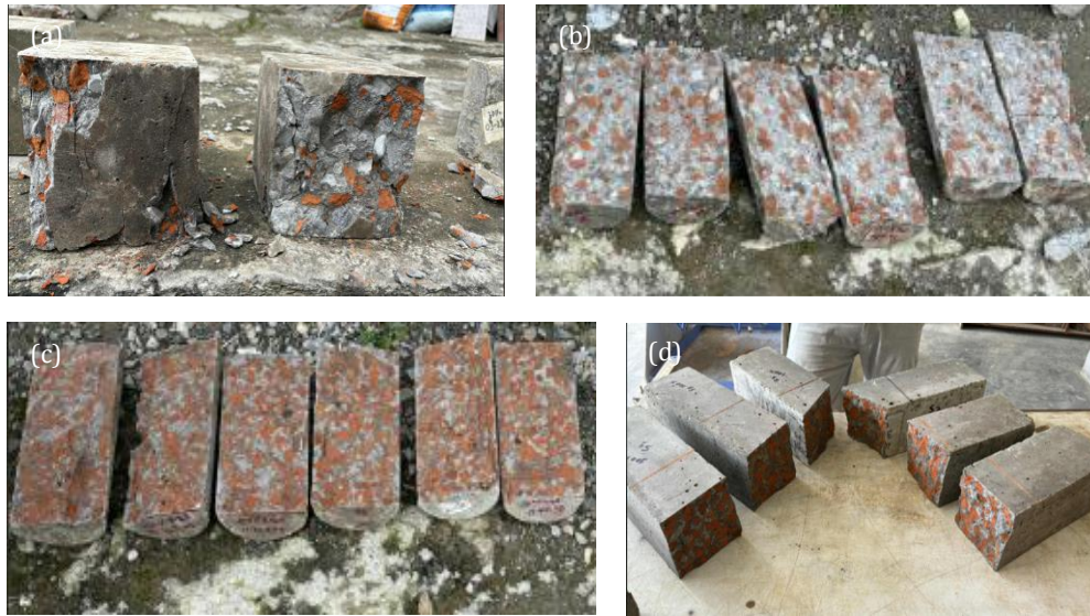
Fig. 14. Failure of different concrete specimens showing cross-section: (a) Cubes of B30%; (b) Cylinders of B30%; (c) Cylinders of B100%; (d) Beams of B100%.
