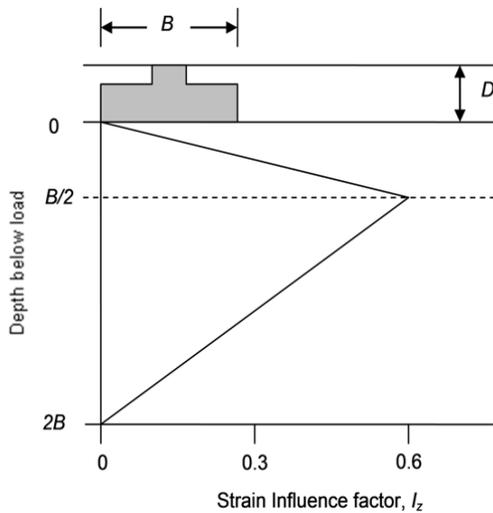
Fig. 1. Variation of strain under a footing (Schmertmann, 1970).
