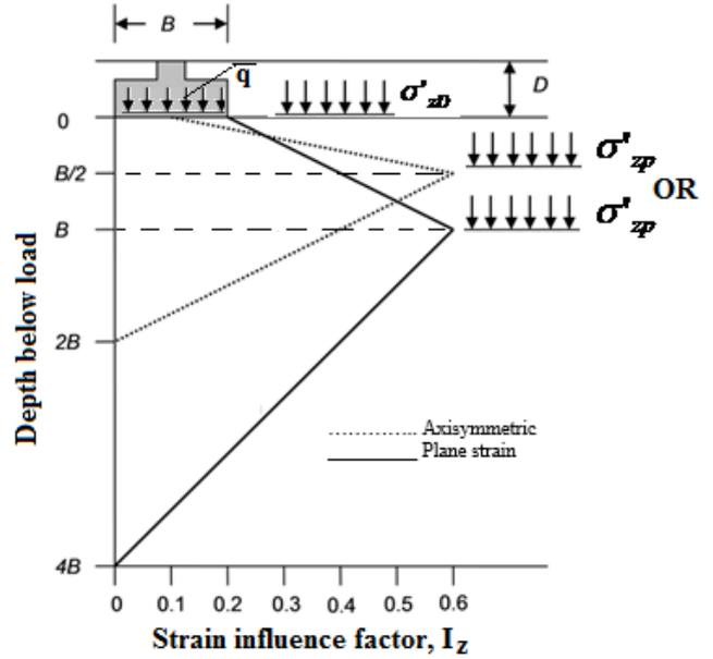
Fig. 2. Strain influence factors (Schmertmann et al. 1978).
