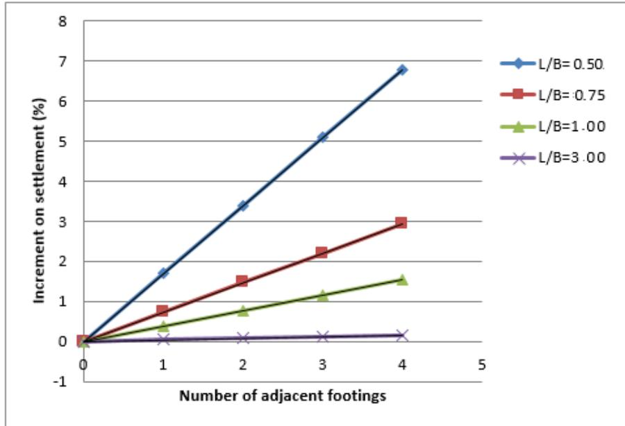
Fig. 5. Increment ratio versus number of adjacent footings.
