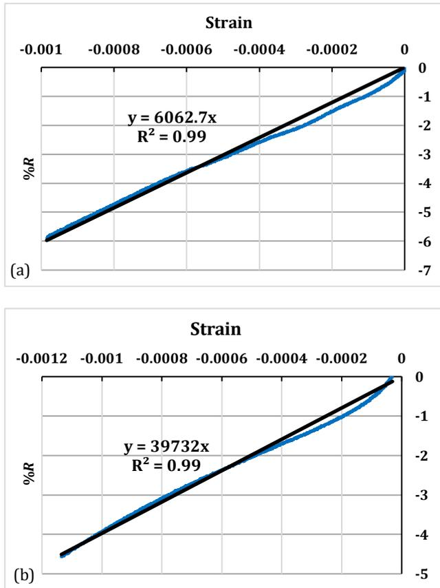
**Fig. 5.** Strain-the percent change of electrical resistance:
