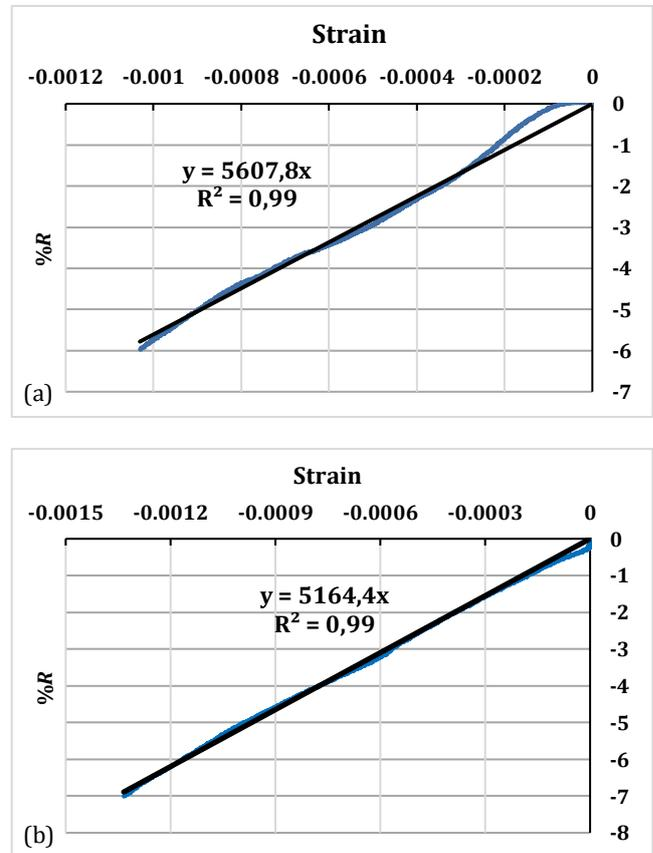
**Fig. 4.** Strain-the percent change of electrical resistance: (a) Br2 (0.5%) mixture ( $K=58$ ,  $LE=8\%$ ,  $R^2=0.99$ ); (b) Br3 (0.8%) mixture ( $K=53$ ,  $LE=3\%$ ,  $R^2=0.99$ ).
