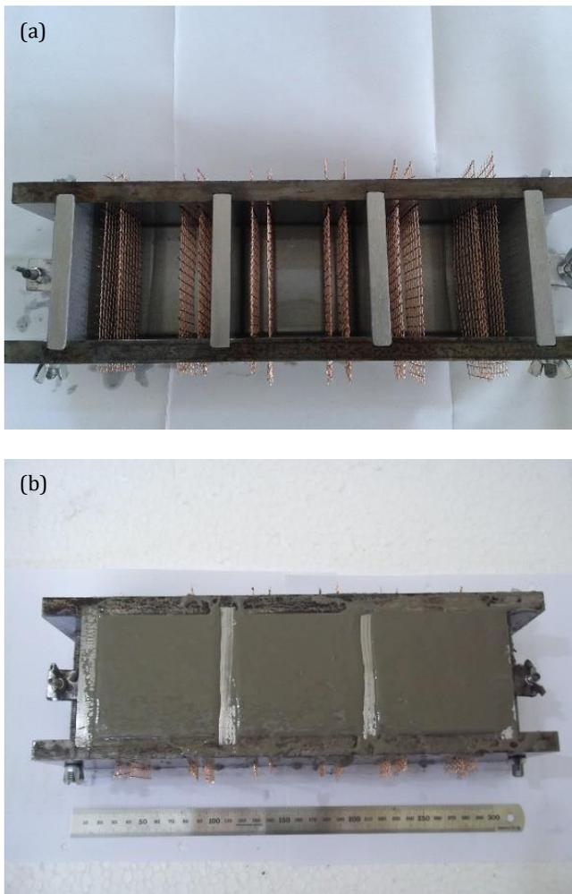
**Fig. 1.** (a) Mold and electrodes; (b) After casting.
