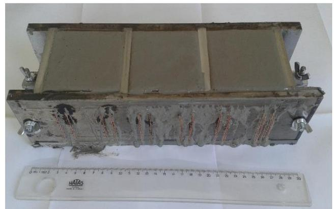
**Fig. 3.** Mix casted in mold.
