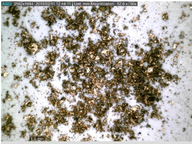
**Fig. 1.** Copper powder microscope image (magnification: 50x).
