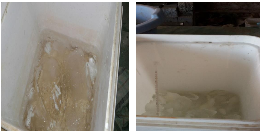
Fig. 1. Crushed ice used for cooling mixing water.
