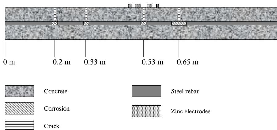
Figure 2. Concrete model, used for FEA with the crack locations
