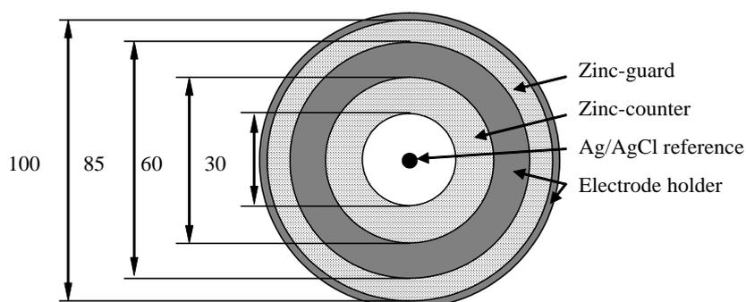
Figure 1. Schematic illustration of the instrument (i.e. GalvaPulse™) using guard ring to limit the polarized area while performing the corrosion measurement.
