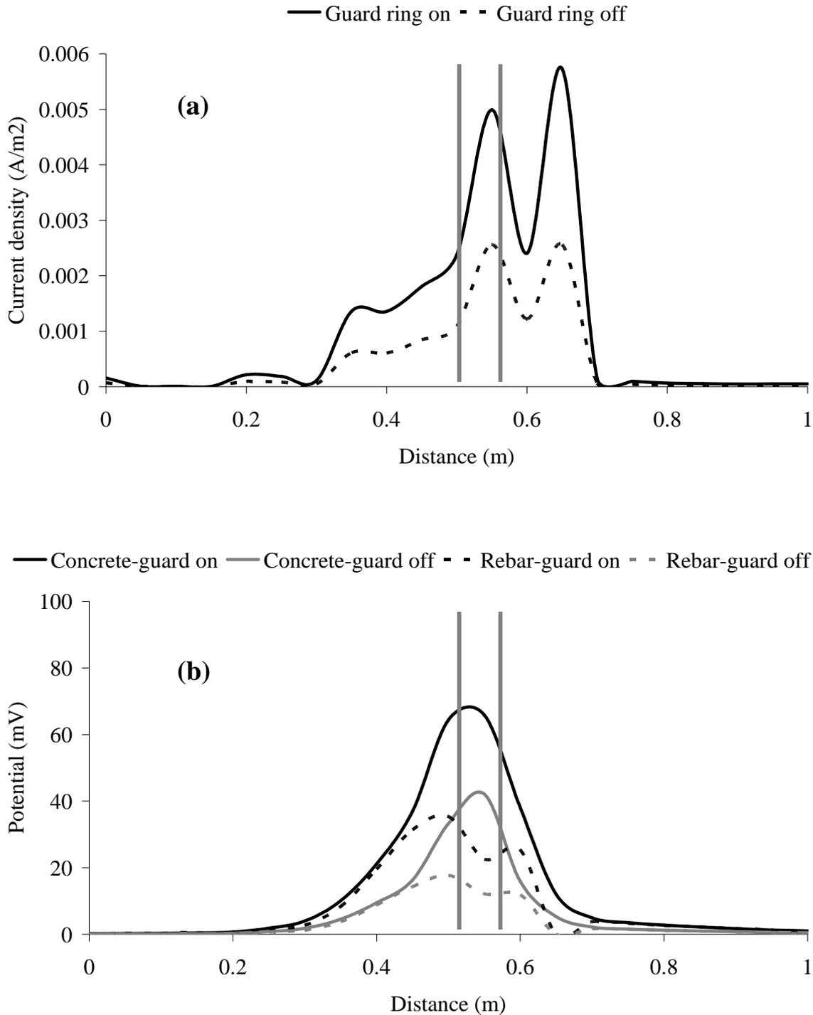
Figure 3. The current density distribution on the steel rebar and the polarization potential distribution on the steel rebar and concrete: (a) rings are on top of the crack location and (b) rings are not on top of the crack location. The vertical grey lines represent the position of the assumed measured area (70 mm)
