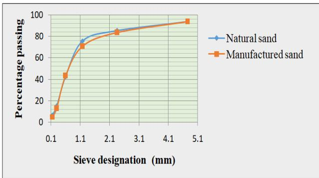
Fig. 8. Grading curve for natural and manufactured sand.
