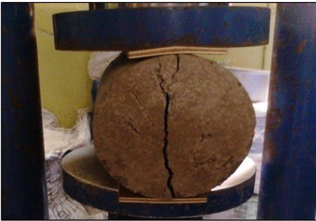
**Fig. 1.** Tensile strength test.
