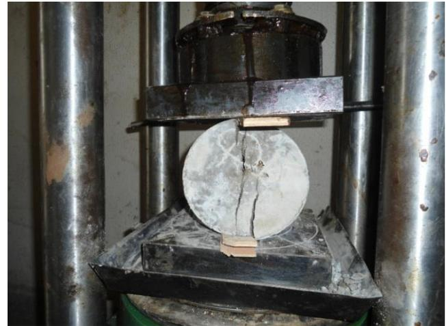
**Fig. 7.** Splitting tensile testing.
