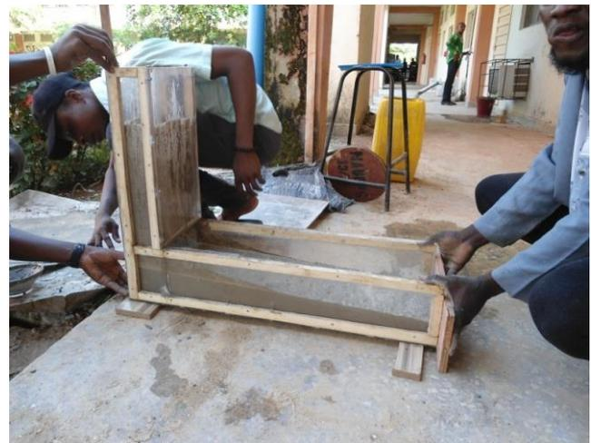
(b) L-box flow test
