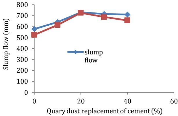
Fig. 5. Slump and J-ring flow values compared.
