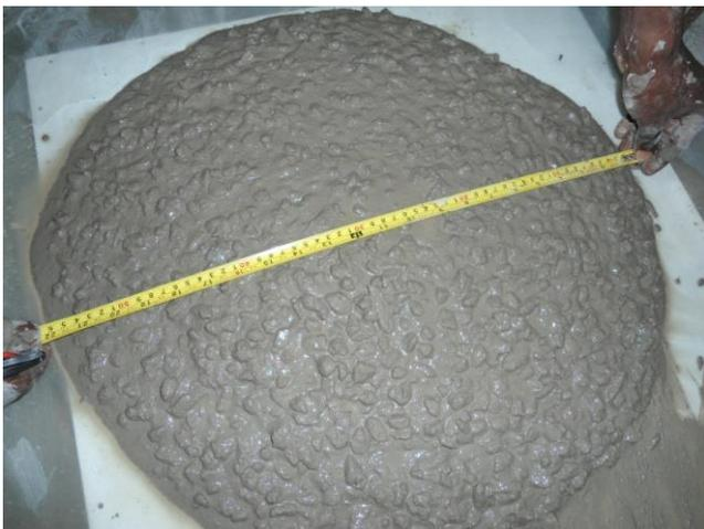
Fig. 1. Slump flow test measurement.
