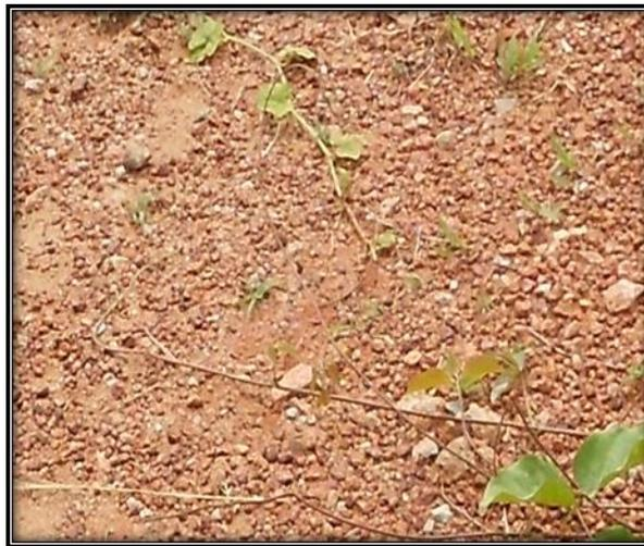
Figure 1. Laterite aggregates on earth surface.
