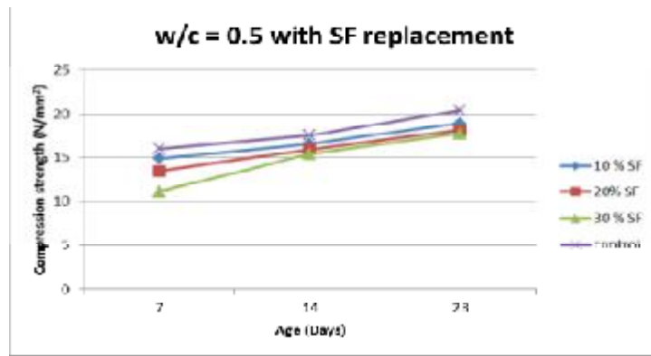
Figure 7. Comparison of compressive strength of mortar with different percentages of SF replacement with OPC mortar (w/c = 0.50).
